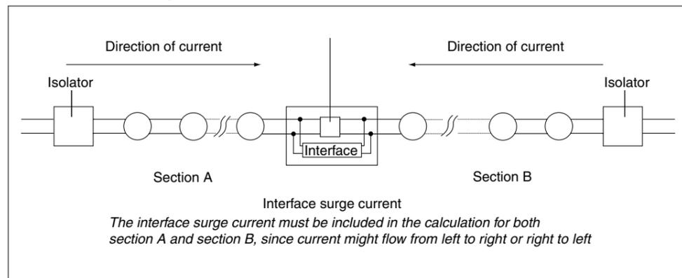
**Fig 1** Diagram to show loading of an isolated loop
